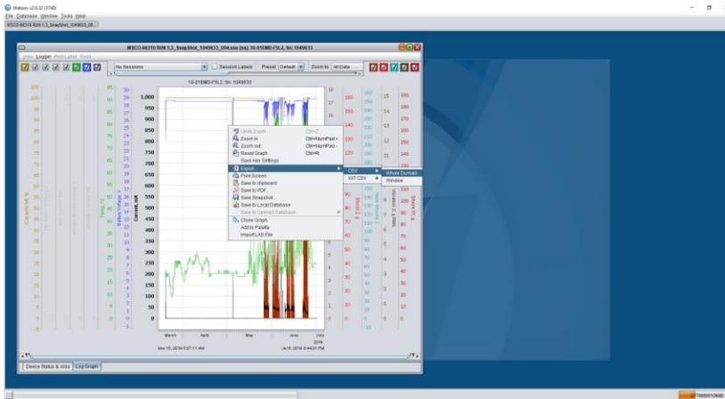
5. Import the newly created CSV file into Wave using the menu Load>>Innova>>Smart-4>>Battery X.
